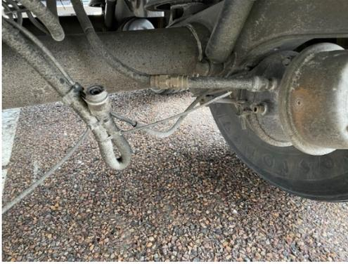
1/30 – Inspector conducted an inspection on a box truck at the I89 Colchester NB weigh station. The inspection revealed a wheel seal was actively leaking on the steer axle of the truck. The truck was placed out of service for the infraction.
