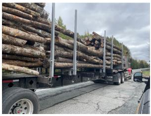
• 10/18 Woodstock, US Rte. An inspector discovered a loose bolt securing the lower fifth wheel halve to the frame. The violation did not meet the out of service criteria.
