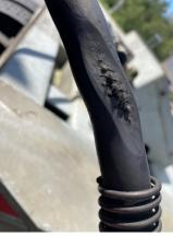
• 9/15, Inspector located a broken leaf in a spring assembly during an Inspection on Rt 103 in Rockingham.
