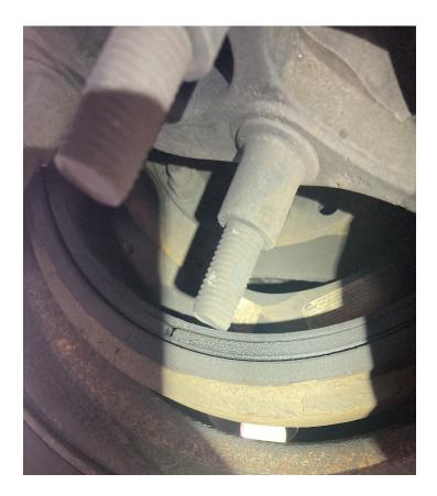
8/17, Inspector performed a level 1 inspection on a truck tractor at the White River Junction detail. An audible air leak on a trailer tire was found (out of service). Two brake pad linings were under <sup>1</sup>/<sub>4</sub> inch (out of service) and two brakes were out of adjustment. The trailer was placed out of service for defective brakes and the flat tire.
