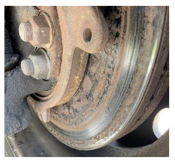
• 7/6, at the WRJ Detail, Inspector performed a level 1 inspection on an intermodal container truck. Both steer axles had cracks in the brake lining and were out of adjustment. Axle 2 had a brake out of adjustment and a loose wheel fastener. The truck was placed out of service for the defective brakes.
