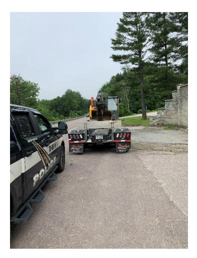
07/05 Morrisville VT Rte 100. An Inspector stopped a CMV transporting a piece of equipment that was not properly secured. The CMV, which in combination required a Class A CDL, was being operated by a Class D licensed driver. An inspection was completed and the driver was placed out of service for not possessing the proper CDL. The CMV was placed out of service for the load securement issue.
