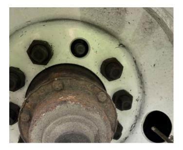
• 7/5, Inspector discovered a rusted brake rotor on a CMV during a level 1 inspection. The driver advised the vehicle had been parked for an extended period of time because the carrier did not have enough drivers.
