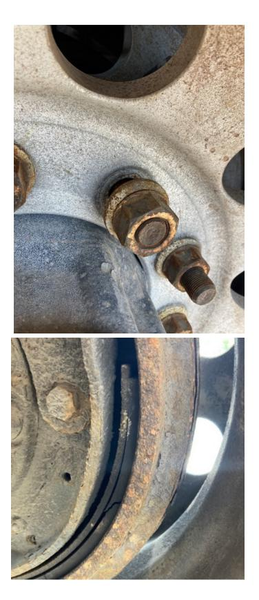
• 7/6, Cpl. discovered brake components hanging from underneath the trailer of an interstate combination vehicle; a slack adjuster had completely disconnected from the brake cam shaft. Additionally, a clevis pin retaining pin was missing from a slack
