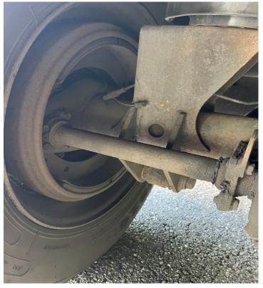
• 6/20, at the Vernon Detail, Inspector performed a level 1 inspection on an intermodal. An improper brake hose splice was found on the trailer chassis. The vehicle was placed out of service until repaired. The truck was missing a bolt in the spring hanger assembly which was documented as a violation.
