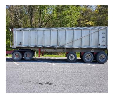
• 5/10, Inspector noticed a tractor trailer combination that had its sliding trailer suspension in the rear most position. The allowable distance from the king pin to the center of the rear most axle group is 41 feet. The distance on this CMV was measured at 44 feet. Additionally, the trailer was placed out of service for inoperable brake lights.
