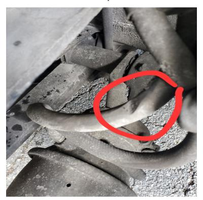
• 4/27, Inspector conducted Level 1 inspection of a truck/tractor hauling large pieces of concrete debris. It was discovered the dump trailer had cracks forming at the hinge point support braces under the trailer. Although a violation it did not meet the out of service criteria.
