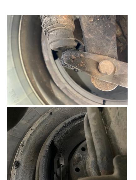
• 4/25, Inspector conducted a Level 1 inspection of a CMV on I91 in Vernon. A front axle brake was discovered to be completely contaminated with grease rendering it inoperable. The truck was placed out of service for the violation. The driver's license was also found to be under civil suspension in Vermont.
