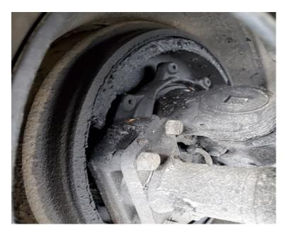
• 4/25, Inspector Stange, conducted a Level 1 inspection of a CMV on I91 in Vernon. The truck was found to have several violations to include a brake hose that was worn through to the reinforcement ply, which caused the truck to be placed out of service. The driver was found to be in violation as well with no ELD on board when it was required and a CDL with a restriction to not operate a Class A tractor/trailer combination. He was also placed out of service.
