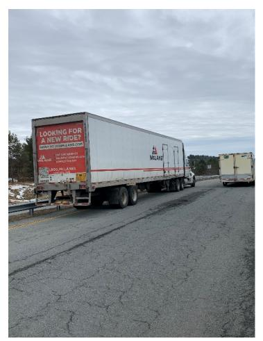
• 04/05 Barton, I 91 N. An Inspector stopped a CMV after observing it was missing a set of dual tires and the axle was secured up using a web strap. The wheel fasteners had failed resulting in the loss of the set of tandem tires that were recovered without incident. An inspection was completed.
