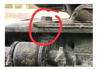
• 4/4, Inspector completed a level 1 inspection of an Intermodal at the Bradford Detail. Brake measurements resulted in all brakes on axles 2 and 3 being out of adjustment, which placed the vehicle out of service.
