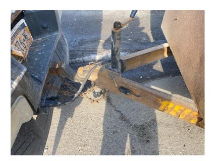
• 3/23 inspected a straight truck at the Williston detail. The inspection revealed building materials were secured improperly on the truck. The vehicle was placed out of service until the driver added necessary strapping.
