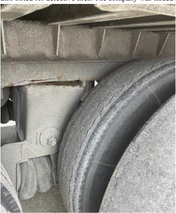
• 03/08, Wells River, US Rte 302. An Inspector conducting a Level 2 inspection discovered a cracked frame and a cracked weld on the fifth wheel pivot bracket. The CMV was placed out of service.
