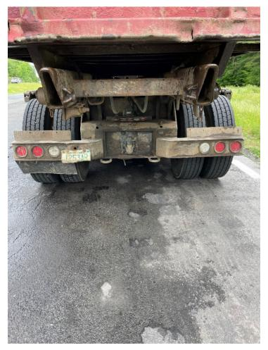
• 6/14, Inspector stopped a dump truck towing an excavator on Route 4 in Woodstock. The driver failed to have the warning flag at the rear extremity of the excavator boom arm that was projecting past the end of the trailer. A loose wheel fastener was found on the trailer. Both were documented as violations and the rear flag was corrected before continuing.
