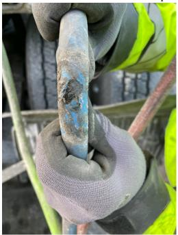
• 12/29, located kinked air lines during an inspection at the WRJ detail.
