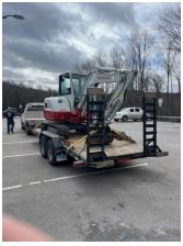
03/19 – An Inspector conducted a traffic stop on a commercial motor vehicle for failing to stop at the open Colchester Weigh Station detail on I-89 in Colchester. An inspection was completed, and the trailer was placed out of service due to the breakaway not attached to the power unit. There were also loose parts of the transported vehicle on the trailer not secured from falling onto the highway.
