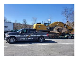
• 3/12, WRJ I91 S rest area, Inspector conducted a Level 2 inspection on a tractor trailer unit. The inspection revealed a kingpin violation on a 53 ft trailer. The maximum distance allowed between rear axles and kingpin was 41ft which measured 44ft on this vehicle. The violation was repaired on scene.
