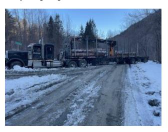
• 3/12, WRJ I-91 S rest area, Inspector conducted a Level 2 inspection of a tractor trailer unit hauling a large excavator. The inspection revealed several permit violations and cargo securement violations. It was discovered the machinery did not have sufficient tie downs for its weight (out of service). The combination was placed out of service until the issue was remedied on scene. A warning was written for the permit violations.
