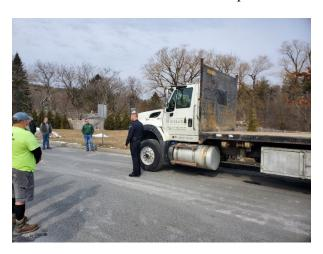
• 2/23, Cpl. discovered multiple lighting violations, a loose 5<sup>th</sup> wheel fastener, and a flat tire on an interstate combination in foreign commerce. The trailer was placed out-of-service for no brake lights, no right rear turn signal and a flat tire.
